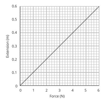
At the elastic limit, the spring will no longer return to its original shape. Once a spring has reached its elastic limit, it no longer obeys Hooke's law.
